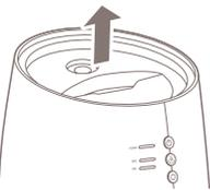
**Caution:** Do not tilt the device when raising the water tank. This may lead to spillage of water remaining in the device.
